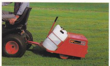
When spiking, fill sprayer tanks to increase weight and improve penetration.
