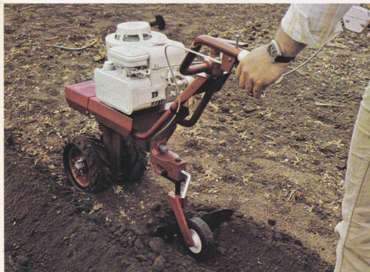
Furrower and Stem using Depth Control Wheel.
